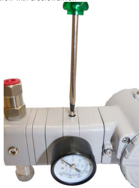
Figure 4.3 – Removing the restriction from the converter
